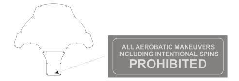
On the instrument panel in pilot's field of vision:
