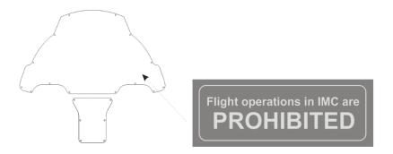
On the instrument panel in pilot's field of vision:
